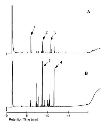
**Fig. 5.** Chromatogram of fatty acid of strain AO01 (A) and strain DO05 (B). Arrows indicate the i-C14:0 (1), i-C16:0 (2), i-C17:1 (3), and 10-Me-C17:0 (4).
